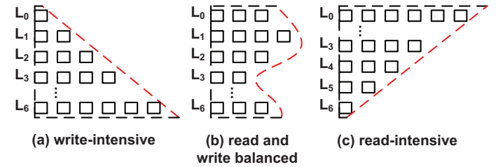
Fig. 3. Adjust LSM-tree shape to adapt to different read and write characteristic workloads.
