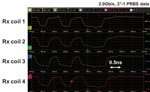
Fig. 5. Bus communication between coils.
